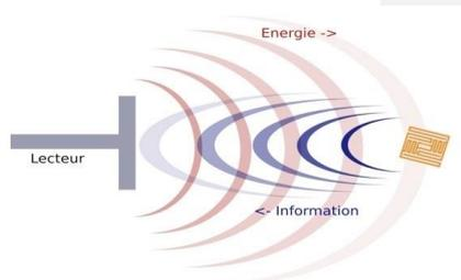
Figure 3 : configuration RFID du Surefeed (Source: Draetta, Delanoë 2009)
